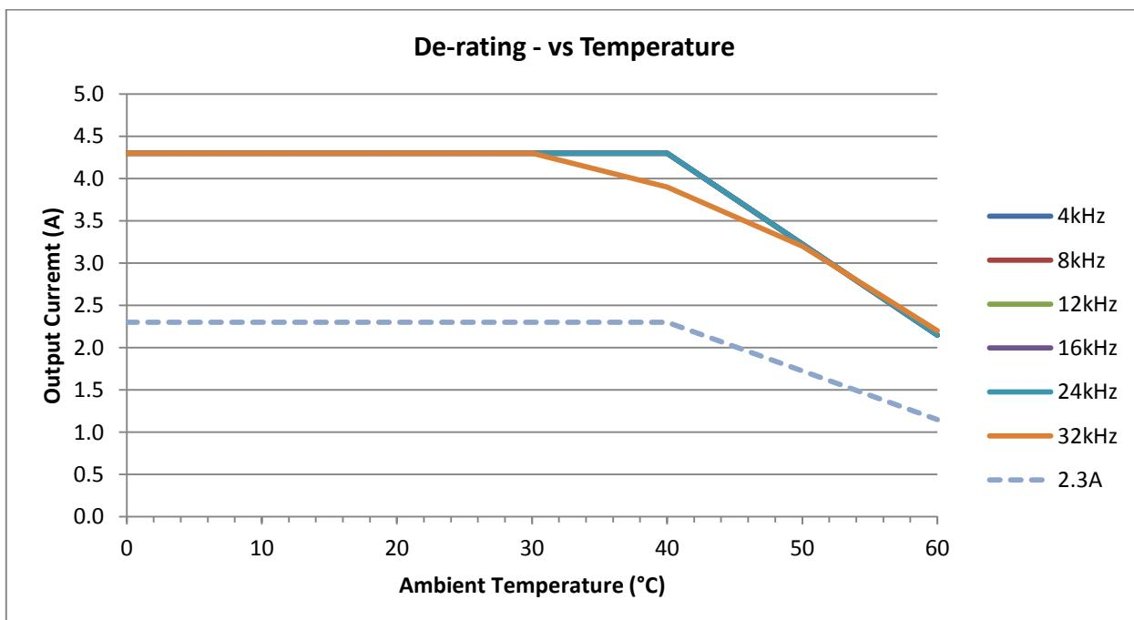
**5.3.2. Size 1, IP20, 200-240V, 2.3A, 4.3A & 7A**
